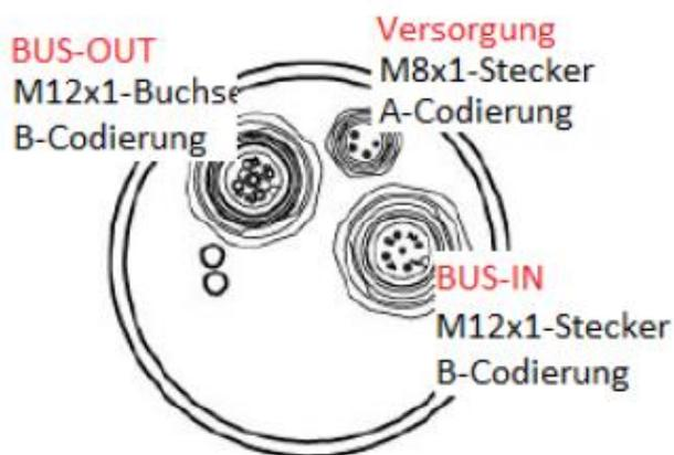
Figure 4.14: DB4 connections - 2x M12, 1x M8
