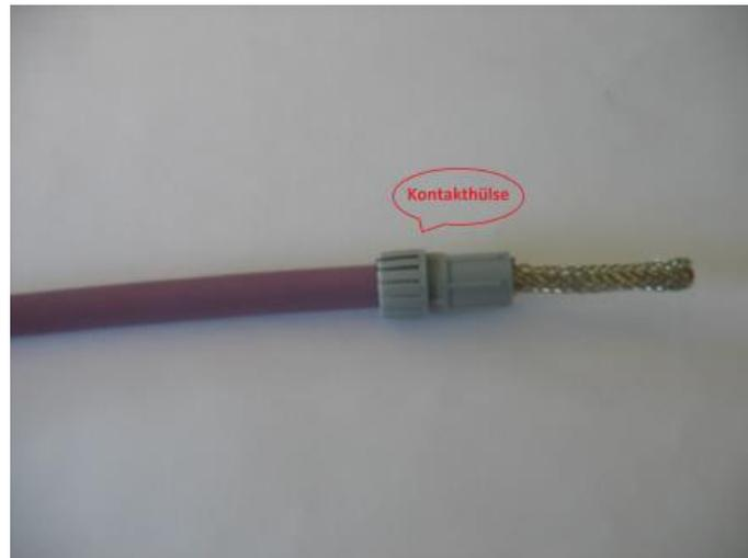
*Figure 4.6: Stripped PROFIBUS standard cable*
