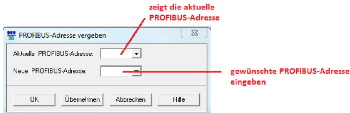
Figure 4.12: Step7 - Assign PROFIBUS address
