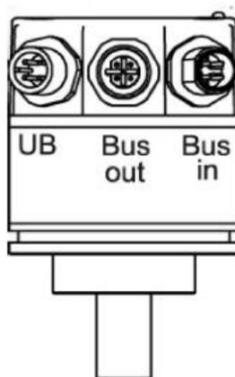
Figure 4.10: BP2 connections - 3x M12
