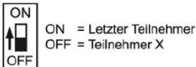
Figure 4.3: Dip switch - Bus cover
