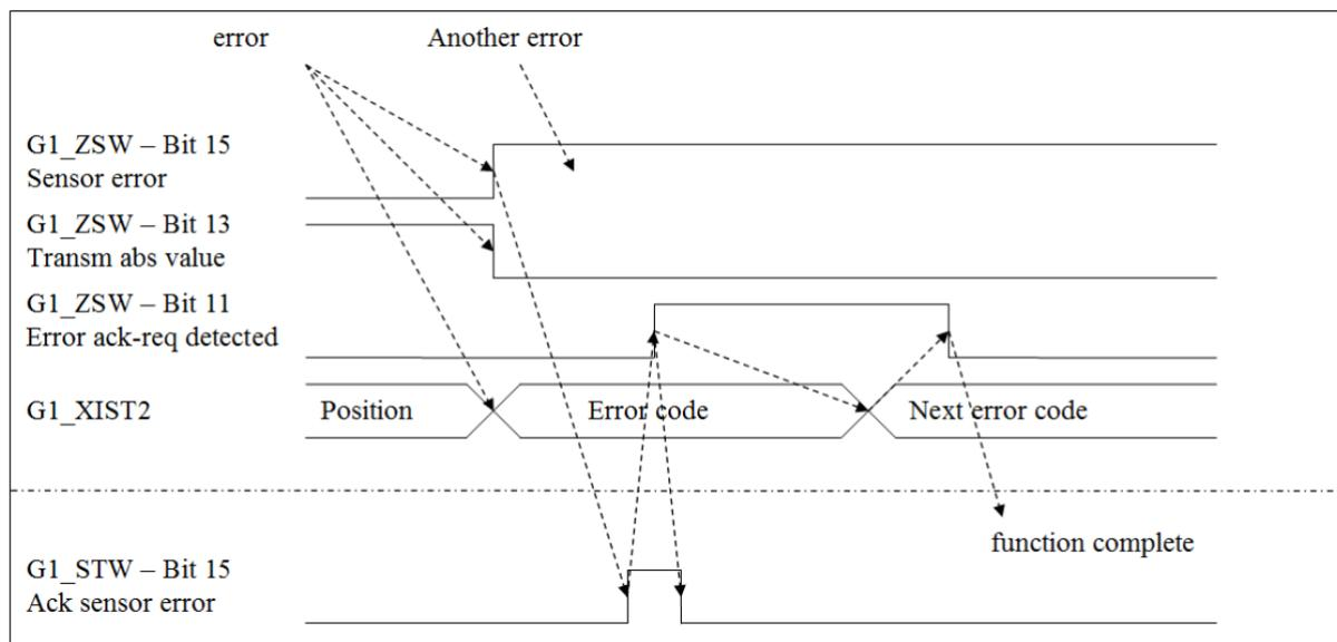
Figure 6.3: State diagram G1\_XIST2 error control - error case
