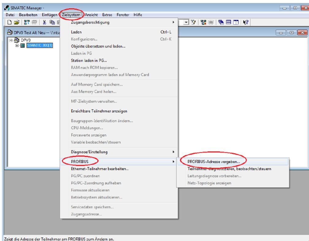
Figure 4.11: Step7 - "Assign PROFIBUS Address..."
