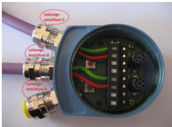
Figure 4.9: Installation example - PROFIBUS standard cable
