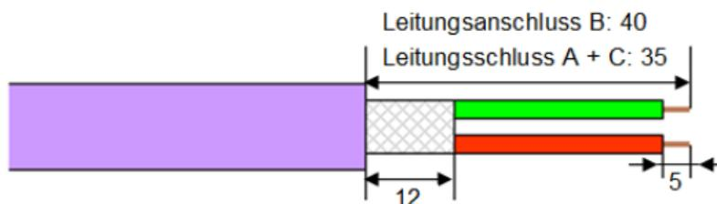
Figure 4.5: Lengths for stripping - Schematic
