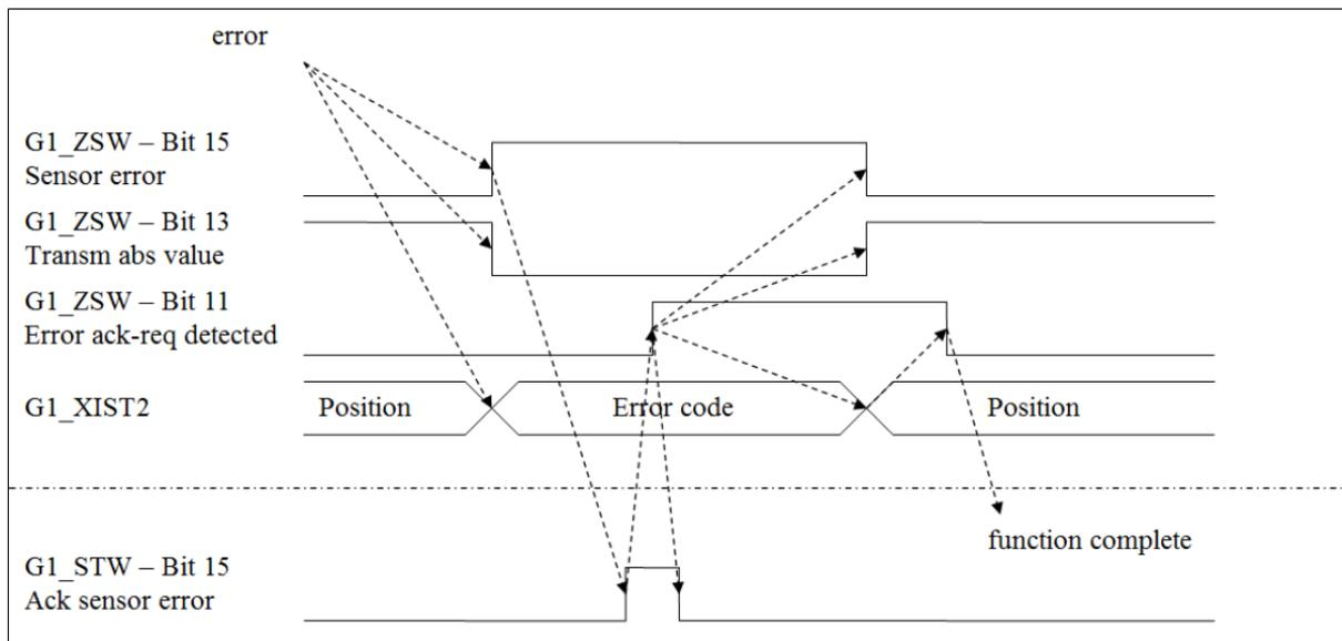
Figure 6.2: State diagram G1-XIST2 error control - error-free case
