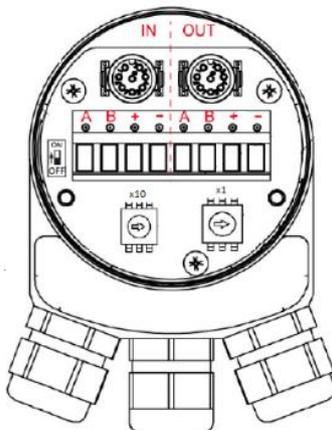
Figure 4.4: BP1 connections - PG screw fitting
