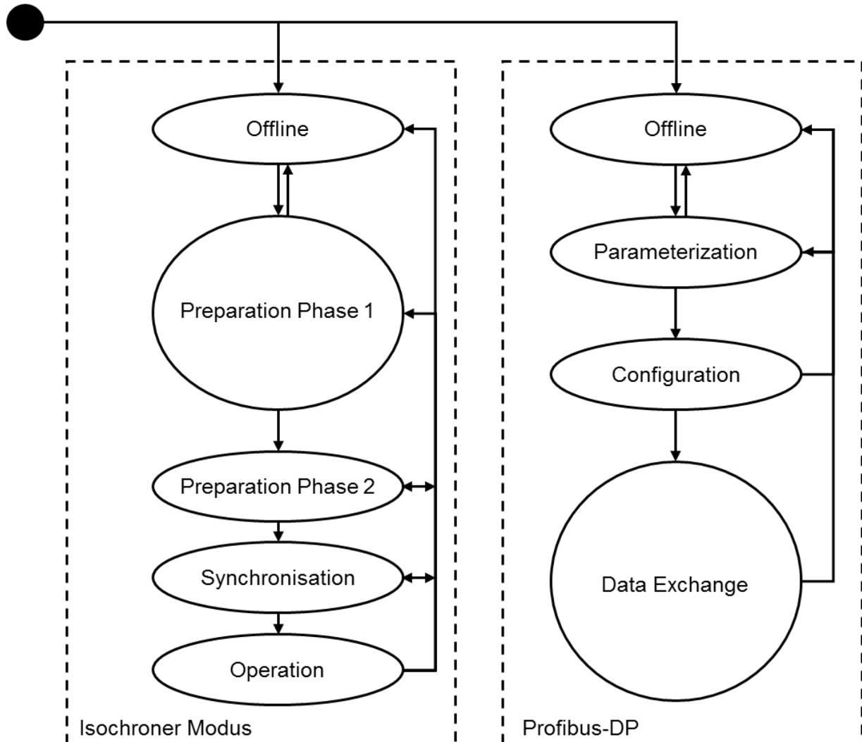
Figure 6.6: Isochronous State Machine and DP State Machine
