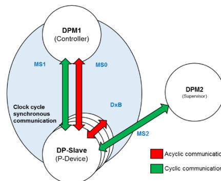
Figure 7.14: Communication Model - Illustration on PROFIBUS-DP
