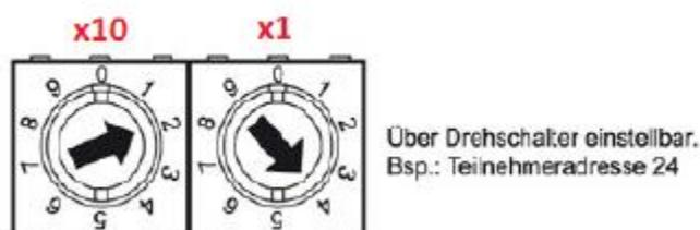
Figure 4.2: Rotary decimal encoding switch - bus cover
