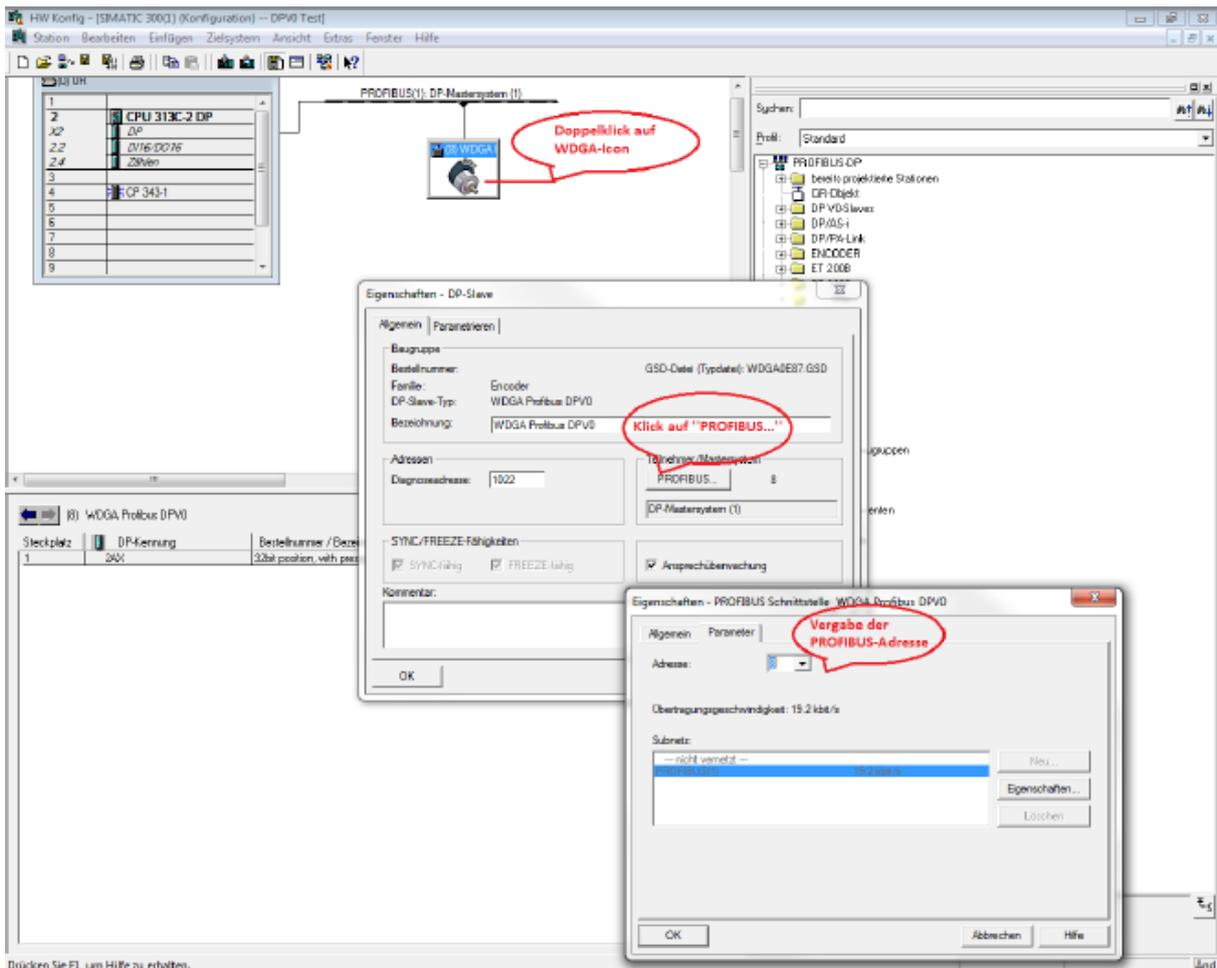
Figure 5.4: Address assignment - "HW configuration" STEP 7
