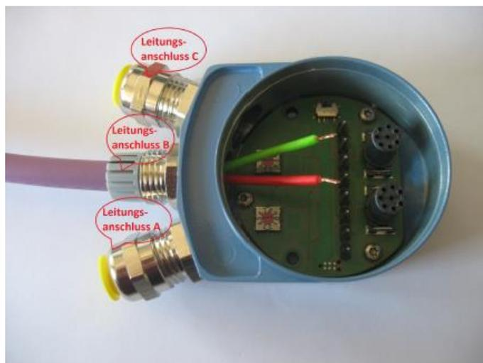
Figure 4.8: Preconfigured PROFIBUS standard cable through PG cable gland
