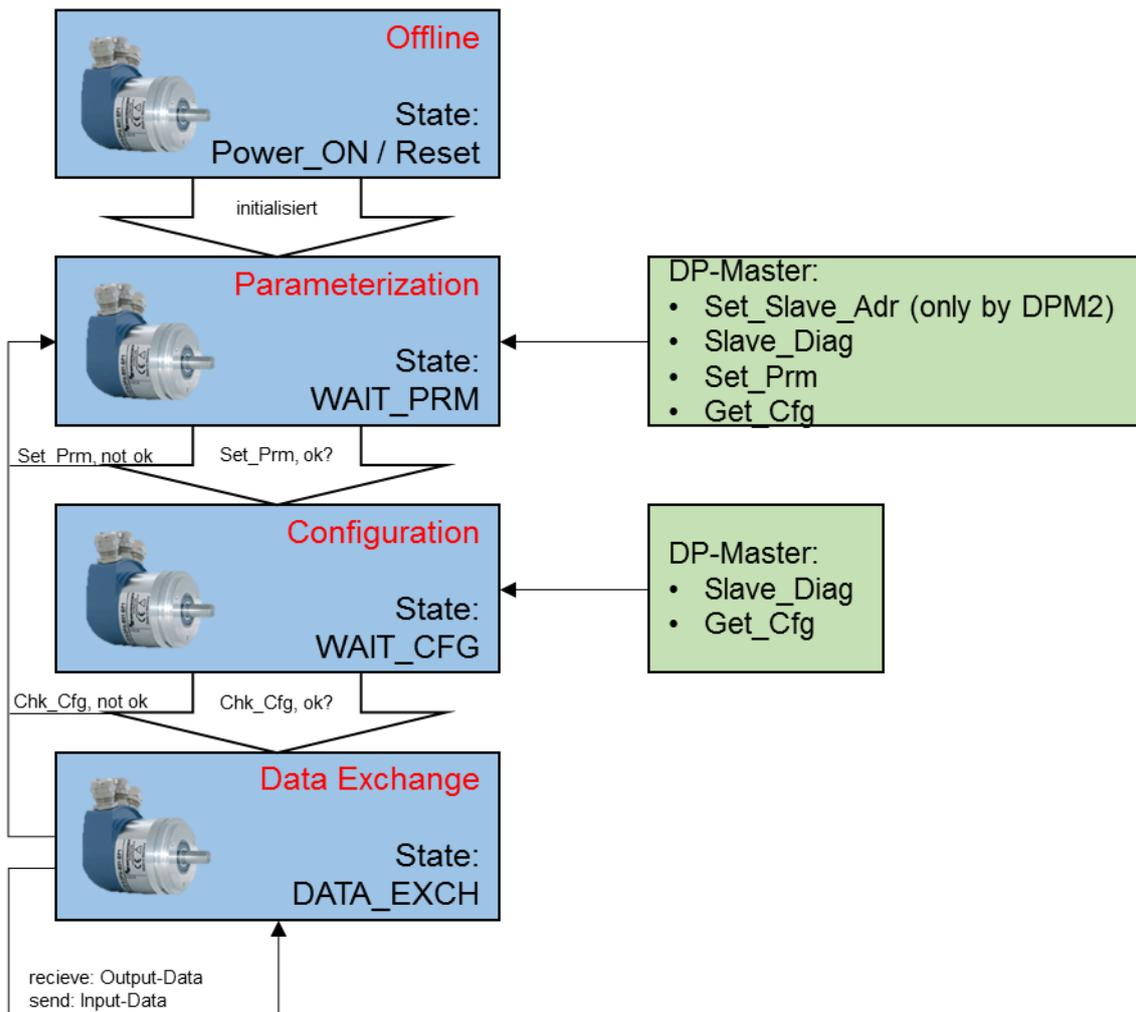
Figure 7.6: State machine - WDGA rotary encoder
